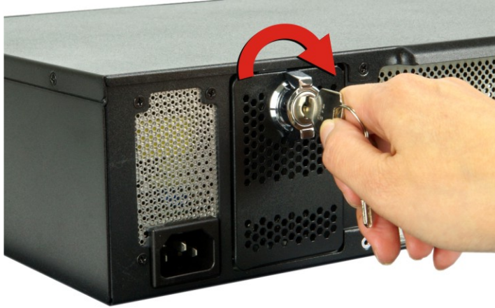
Figure 3-1: Unlock HDD Cover
